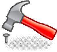
*Hammers* — A hammer blow should be struck squarely and parallel to the surface being struck. Glancing blows can cause injury. Never use a hammer with a loose or damaged head or handle. Look for dents, chips, cracks, or other signs of wear and tear. Use riveting hammers for sheet steel, carpenter or claw hammers for driving and pulling nails, and ball-peen hammers for metal work.
